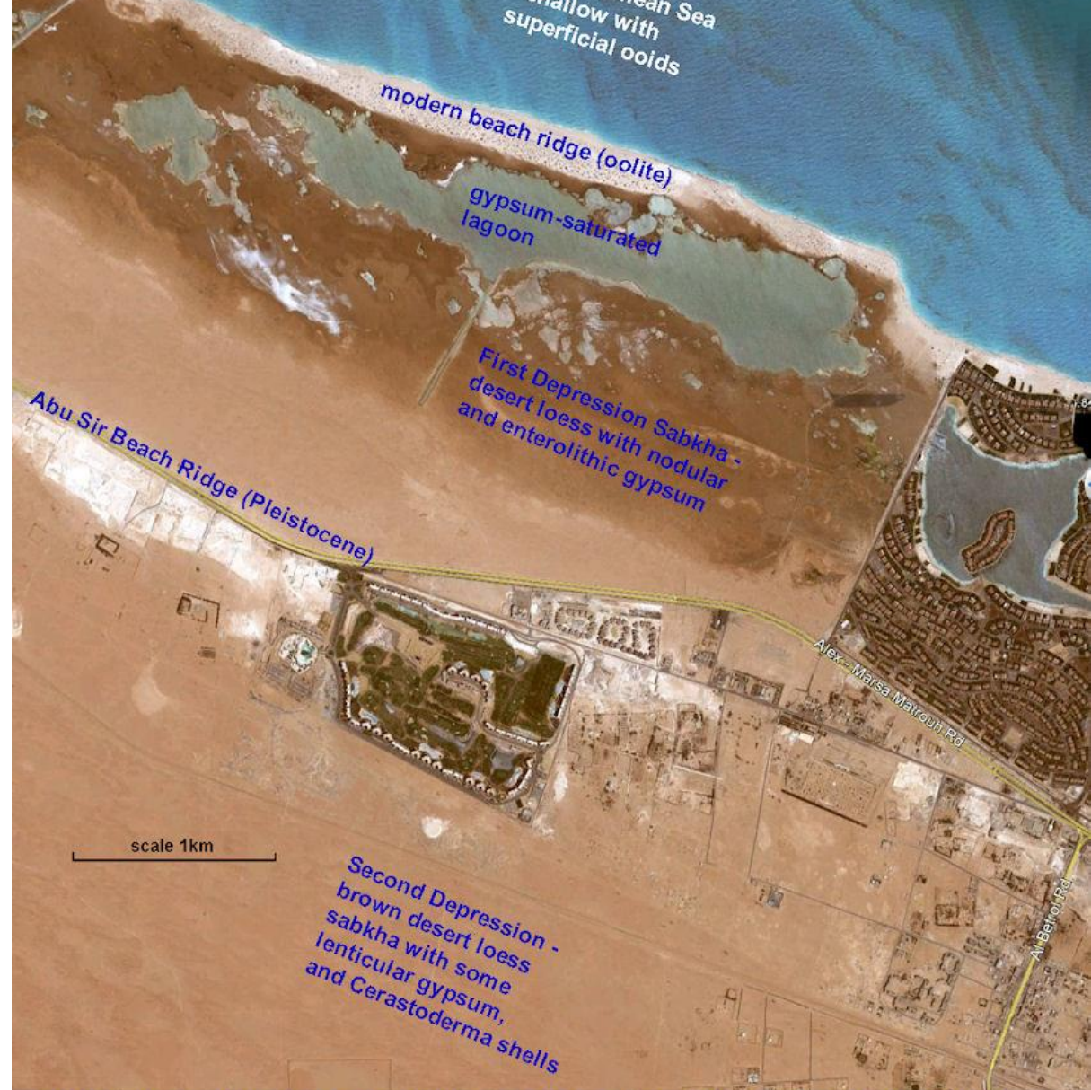
A GYPSUM-SATURATED LAGOON IN THE FIRST DEPRESSION AT EL ALAMEIN, EGYPT. This lagoon remains in natural condition. Others further east have been altered and developed since the area was studied in the late 1970s (notice hut development at the right). Gypsum was found to be precipitating at the margin of this lagoon. There is a little halite as a surface crust to the SW of the lagoon. The beach is mostly white oolitic sand. The road is on the Abu Sir Ridge, a calcrete-cemented, Pleistocene beach ridge. Aerial photograph modified after Google Earth, 2011. Ian West.
