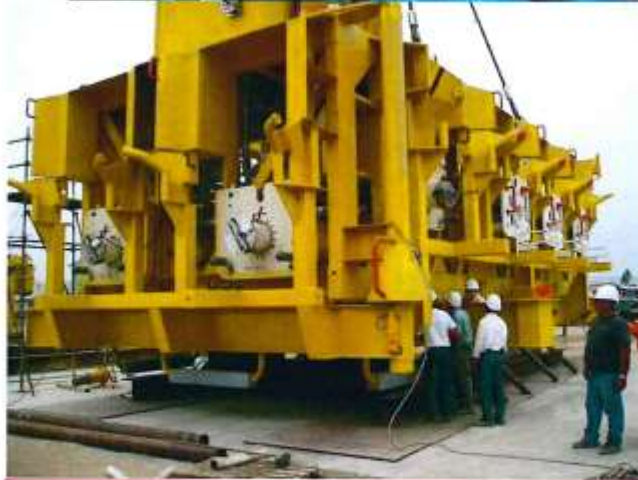
Manifold Module Capable of accepting Pigging Loop Module
