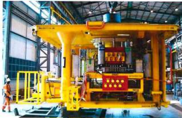
Drill Through Horizontal Christmas Tree Capable of accepting multiphase flowmeter
